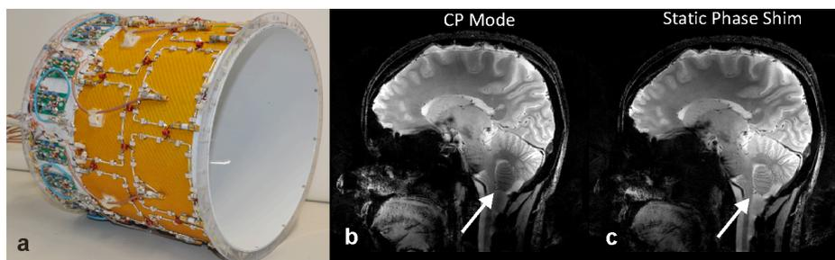
Fig. 1: (a) Dual-row 16-channel transceive / transmit array for imaging at ultra-high fields. (b and c) Performance record: The use of static phase shimming (c) features homogenous excitation of the entire volume in comparison to images taken in conventional CP mode (b) featuring dark areas indicative for inhomogeneous excitation.
