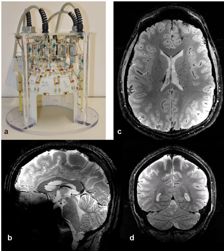
**Fig. 2:** (a) Receive array optimized for MR imaging the human brain. (b, c, d) Performance record: In-vivo images with high SNR and whole brain coverage.
